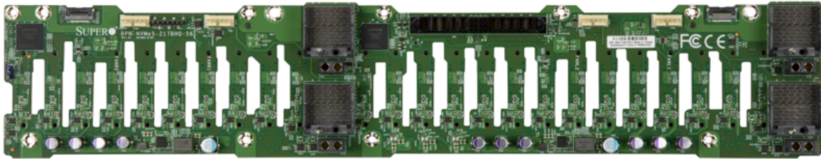
Figure 3-42. SATA/NVMe Backplane (Side Facing Chassis Rear)
