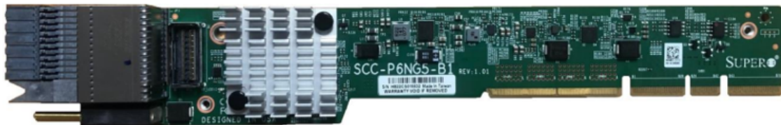
Figure 3-44. Storage Adapter (SCC-P6NG5-B1)
