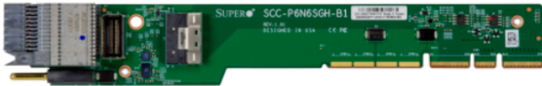
Figure 3-43. Storage Adapter (SCC-P6N6SGH-B1)
