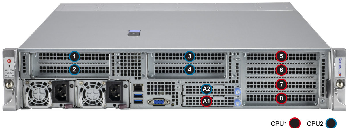
Figure 3-43. Expansion Card Chassis Slots
