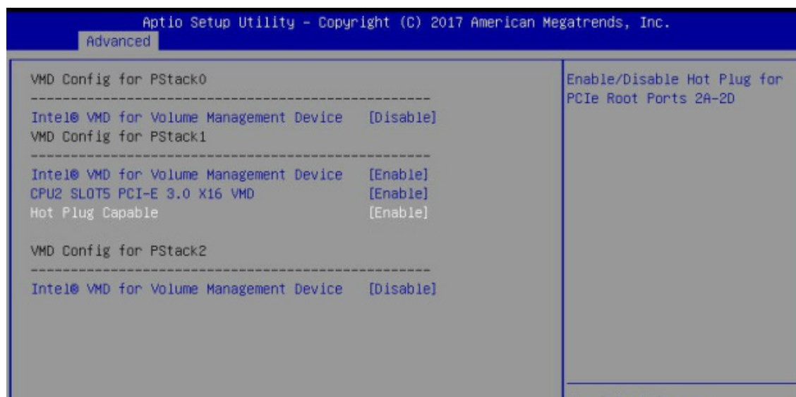
Figure 6-7. BIOS, Enabling CPU2 Example
